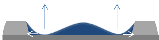
Figure 11. A schematic showing how evaporation (blue arrows) and capillary suction (white arrows) thinned the film in intermediate regions and prevented capillary flows coming from the centre of the fluid.
