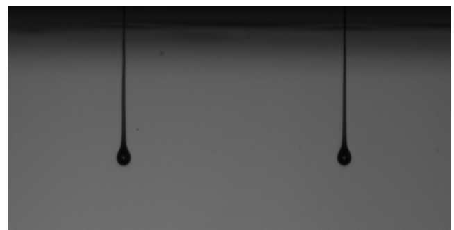
Figure 3 - Drop Formation, Single Event Imaging (JetXpert)
