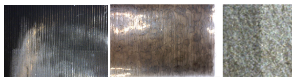
Figure 7. Inkjet printed samples on different substrates: from left 1) water based ink on Nafion film, 2) solvent based ink on Nafion film, 3) water based ink on carbon paper (darker area on left).
