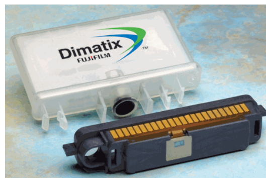
Figure 2: Dimatix piezo-based printhead/jetting device. [2]
