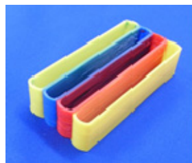
Figure 13 Sample product using 4 filaments with multiple nozzle line-type printhead
