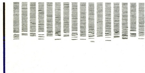
Figure 8 Nozzle Health Pattern With Missing/Clogged Nozzle in Lower Half of the Nozzle Swath
