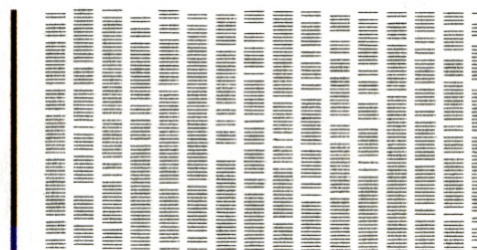
Figure 9 Nozzle Health Pattern with Missing/Clogged Nozzle Randomly Scattered
