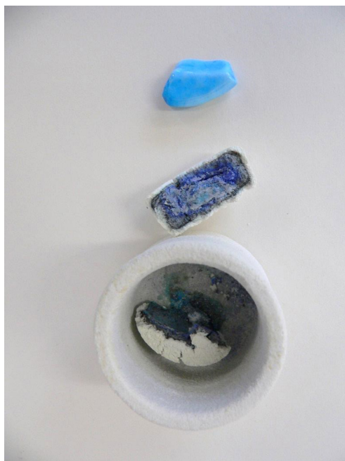
Figure 6: Fused silica test piece fired in glaze powder GP1c
