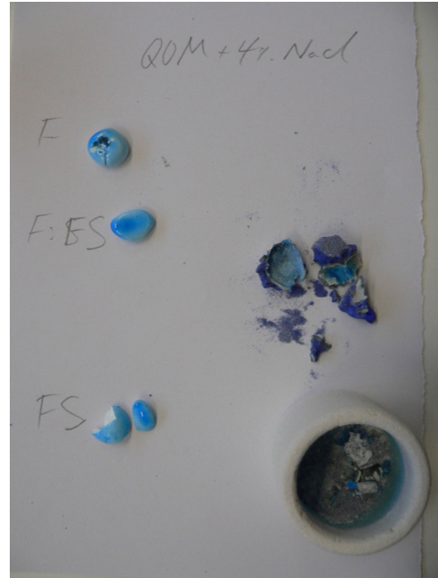
Figure 5: Fired test pieces cementation glazed with GP1b
