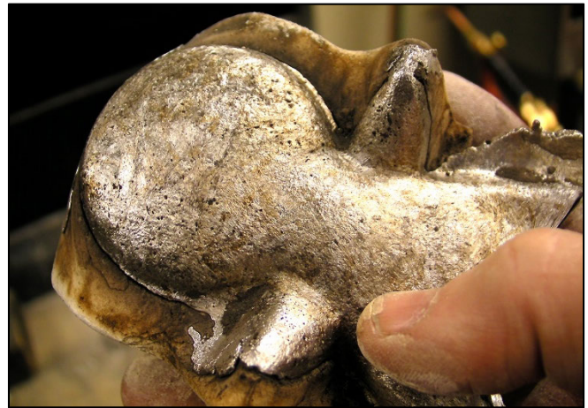
Figure 10: Printed mould and cast aluminum
