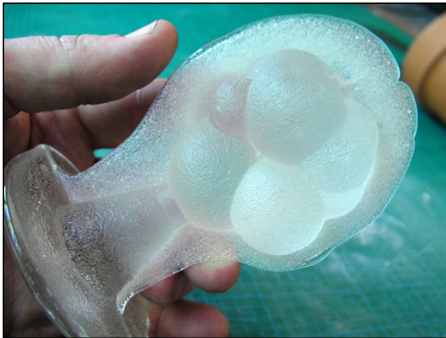
Figure 16: Surface detail, form and seam flashing, post-casting
