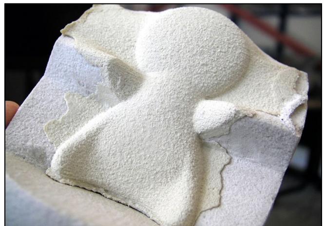
Figure 11: Printed mould and slip cast ceramic
