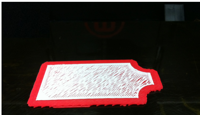
Figure 2. 3D Printed specimen one layer of PLA at 45°.
