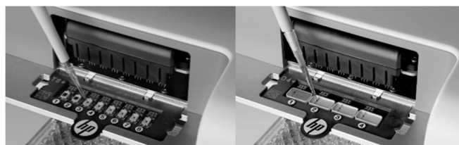
Figure 3: Pipetting into the 10 \mu\text{L} T8 cassette [left]; Pipetting into the 200 \mu\text{L} D4 cassette [right]
