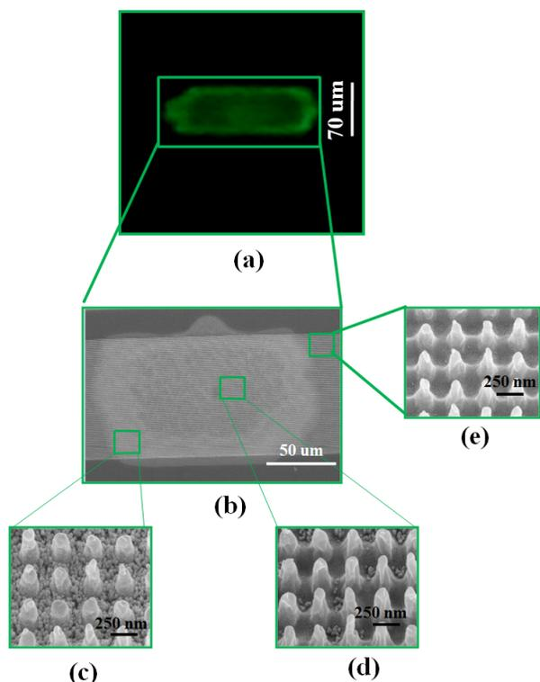
**Figure 3.** Silver ink printed with bright silver mode on hydrophilic surface. (a) Optical microscope image of one printed dot on green pixel band after laminating the sample. (b) SEM images of the silver dot printed on the hydrophilic surface and (c), (d) and (e) are inset images to show details in different regions.
