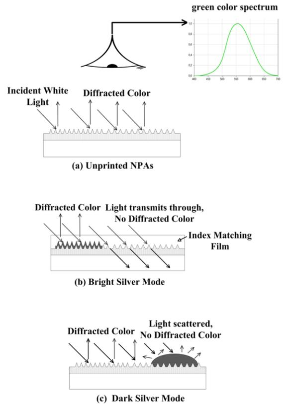
**Figure 2.** Schematic of bright silver mode and dark silver mode for printing colors on NPAs. *(a)* Unprinted NPAs and schematic of the diffraction colors. *(b)* NPAs printed with bright silver mode in which the pixel under the printed silver dot is activated while other regions are deactivated by lamination. *(c)* NPAs printed with dark silver mode in which the pixel under printed silver dot is deactivated while other unprinted regions remain active in diffracting light.
