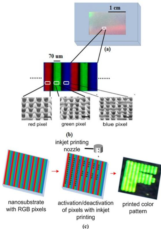
**Figure 1.** Schematic of inkjet-printed OVDs on nanopillar array pixels. *a)* The configuration of a nanosubstrate. *b)* Scanning Electron Microscope (SEM) images of the nanopillar array pixels. The length of scale bar is 500 nm. *c)* Schematic process to print a color pattern on the nanosubstrate by selectively activating or deactivating pixels.
