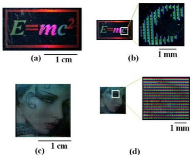
**Figure 6.** Photographic images of printed samples. (a) Color patterns printed with bright silver mode. (b) Zoom-in image of (a) to show the details on the printed color letter 'C'. (c) Color photo printed with dark silver mode. (d) Zoom-in image of (c) to show the details on the eye.
