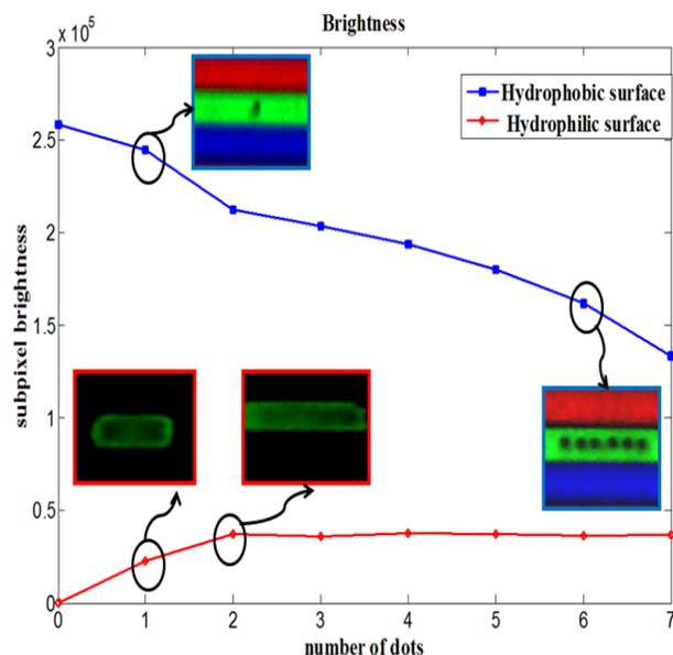
**Figure 5. Effective subpixel brightness v.s. number of printed silver dots on hydrophilic and hydrophobic surface. The inset optical microscope images show the patterned subpixels in the corresponding data points.**
