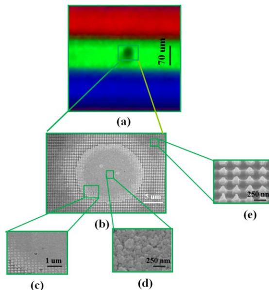
**Figure 4.** Silver ink printed with dark silver mode on hydrophobic surface. (a) Optical microscope image of one printed dot on green pixel band. (b) SEM images of the silver dot printed on the hydrophobic surface and (c), (d) and (e) are inset images to show details in different regions.
