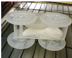
Figure 2. A small "push-toy" car created by a single print on a 3D Systems ProJet® 3500 a) out of the printer, b) melting the support material away, c) final functional car produced in a single build with no assembly.
