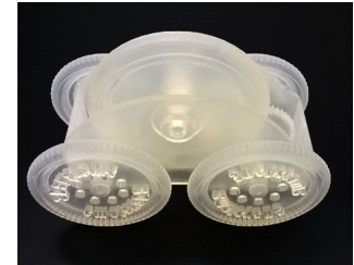
Figure 2. A small "push-toy" car created by a single print on a 3D Systems ProJet® 3500 a) out of the printer, b) melting the support material away, c) final functional car produced in a single build with no assembly.
