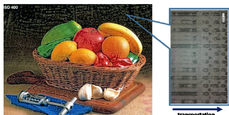
Figure 2 Streaky Image by Dots Coalescing
