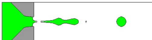
Figure 16 Simulation of the ink ejecting by newly developed driving waveform and pressure chamber
