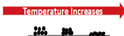
Figure 3. Schematic representation of toner fusing steps as a function of temperature. A good fusability requires toner to melt rapidly as temperature increases.
