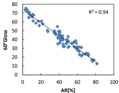
Figure 8. Model that predicts the gloss based on the area ratios of the two image structures.  $60^\circ$  Gloss is the specular gloss at an angle of 60 degrees, and AR is defined as the sum of the area ratio of both the micro hollow and the macro hollow.  $60^\circ$  Gloss =  $73.5 - 0.732 \times \text{AR}$ .
