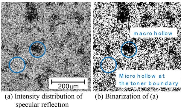
Figure 7. Measurement results of the intensity distribution of the specular reflection on the printed image surface
