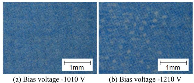
Figure 6. Non-uniformity of the quantity of developed toner particles caused by irregularity of the surface potential on the photoreceptor due to fluctuation of electric discharge. The image shows the output image by roller charging with DC voltage. The white area indicates the exposed paper surface among toner [7].
