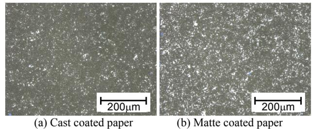
Figure 5. Non-uniformity of the quantity of transferred toner particles caused by irregularity of the electric field corresponds to surface unevenness on the paper. The white area indicates the exposed paper surface among toner. (a) Toner transferred on a cast coated paper. (b) Toner transferred on a matte coated paper.
