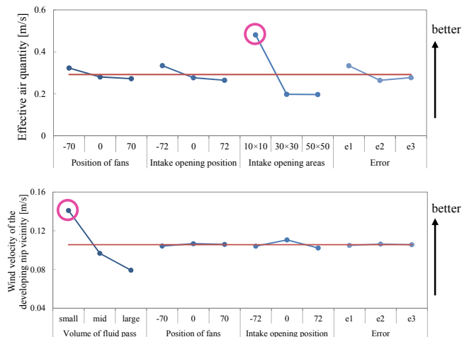
Figure 4. Functional effect diagram of airflow systems (Top: Airsys1, Bottom: Airsys2)
