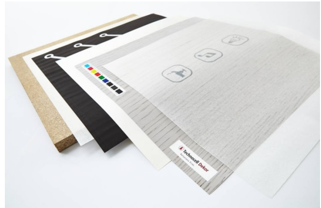
Figure 1. Arrangement of the printed and impregnated décor paper sheets on a chip board substrate before contacting and hot-pressing
