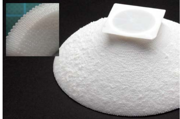
Figure 7. An image of the bobbled texture and a macro photo of wall thickness inset.
