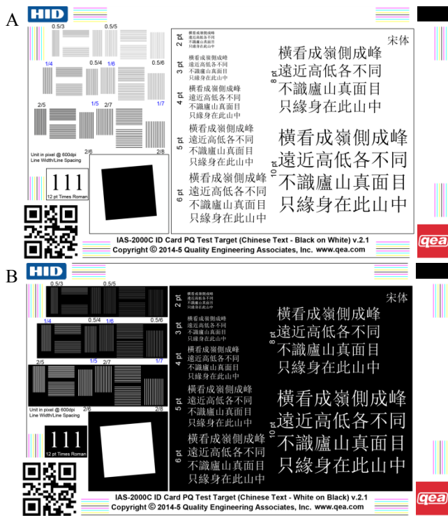
Figure 1. Test Targets for evaluating Chinese text quality, including black text on white (A), white text on black (B).
