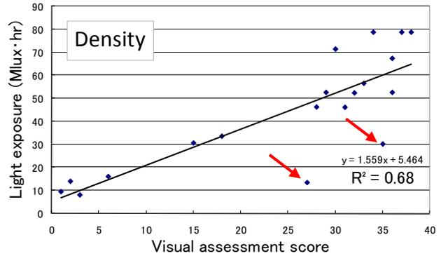
Figure 5a) Visual assessment score vs. amount of light exposure required to reach endpoint stipulated with density criteria.
