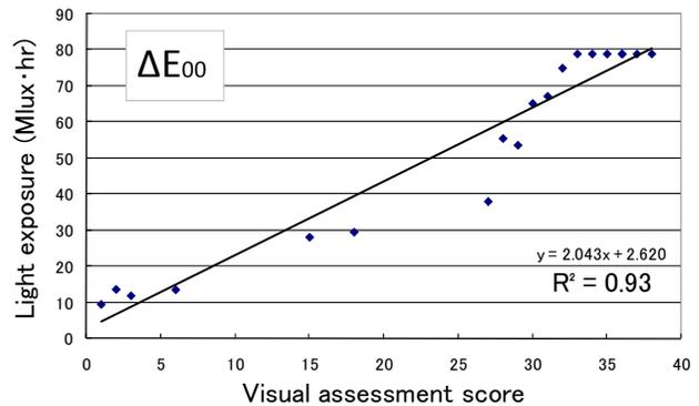
Figure 5c) Visual assessment score vs. amount of light exposure required to meet endpoint  $\Delta E_{00} = 5$ .
