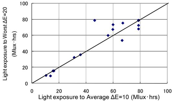
Figure 3 Light exposure required to reach average  $\Delta E$  vs. light exposure required to reach worst  $\Delta E$  endpoints for 22 patches in each material.
