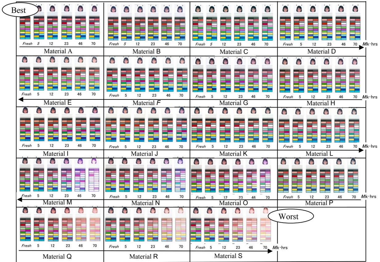
Figure 1 Overview images of the light fading test results of 20 materials. For each material, fresh, 1, 2, 4, 6, and 8 weeks from the left to the right. The materials are rearranged from the best (upper left) to the worst (lower right)
