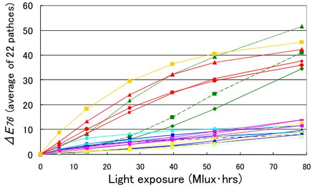
Figure 2 Light-fading test results for 20 samples expressed as average  $\Delta E_{76}$  for 22 patches.
