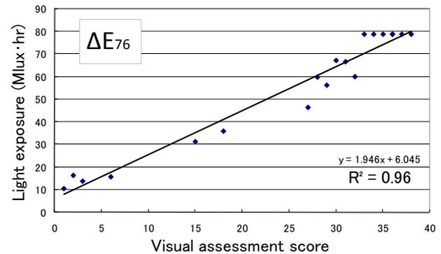
Figure 5b) Visual assessment score vs. amount of light exposure required to meet endpoint  $\Delta E_{76} = 10$ .
