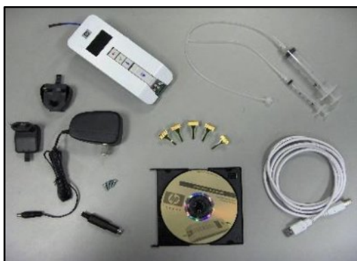
Figure 3. HP® Thermal inkjet pipette system (TIPS).
