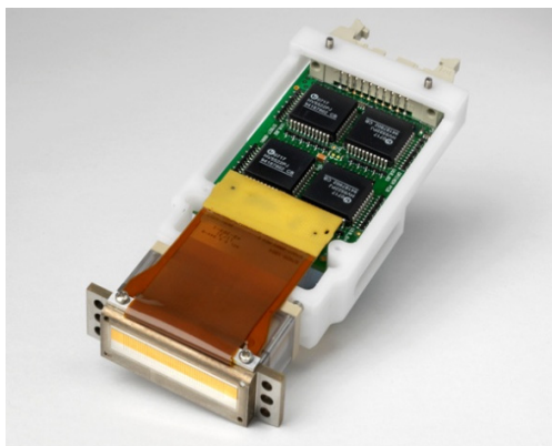
Figure 4: a laboratory prototype of an industrial inkjet printhead with TTP's moving nozzle technology, including drive electronics.
