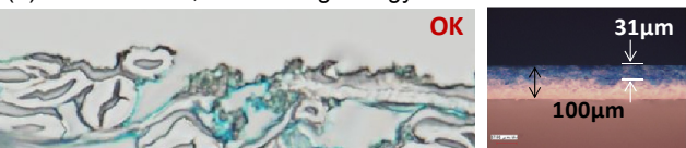
Figure 10. Distribution of pigment in cross-section of printed paper (resolution:1200dpi, drop volume 4.3pl, coverage 100%)
