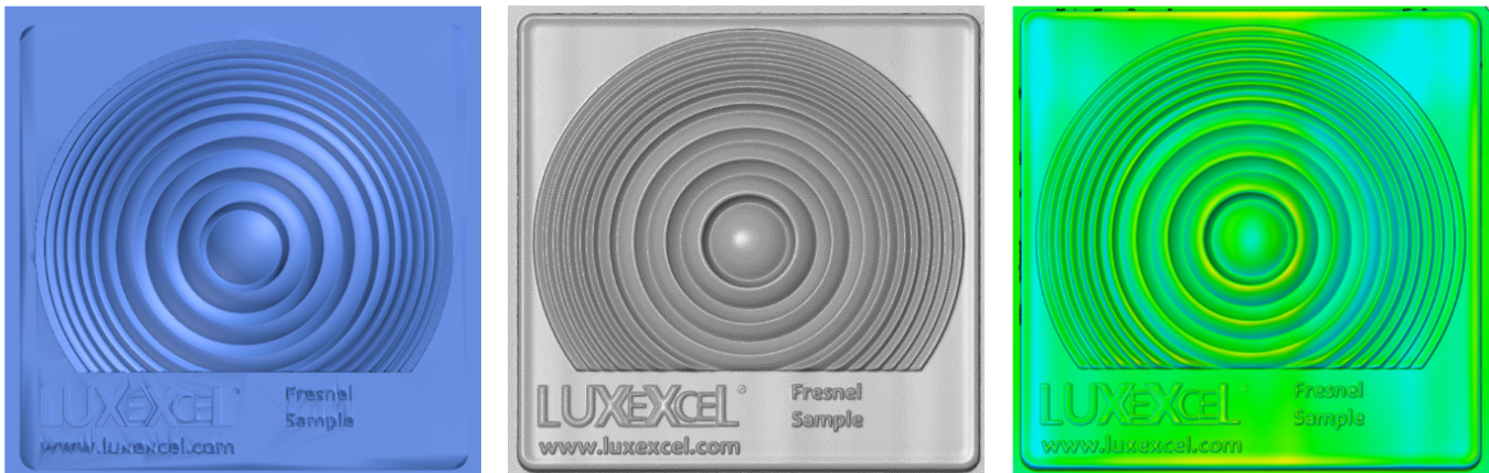
Figure 3: Design (left), measured 3D optic (middle), deviation from geometry (right)
