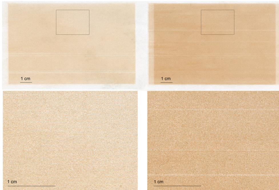
Figure 17. Printed patterns obtained for a substrate speed of 1.0 m/s, 13.1 pL droplets, and 5 mm gap (left: one row; right: two rows). The substrate motion was toward the right. Bottom: the delimited regions are displayed in more detail.
