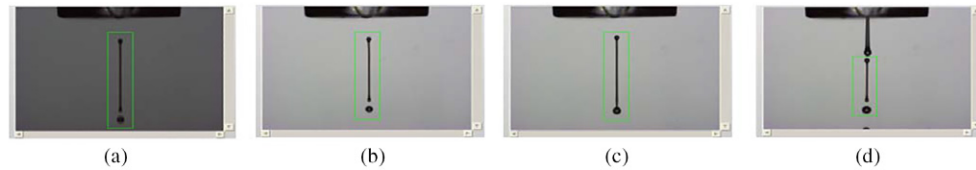
Figure 13. Droplet images for the mixed ink with IPA and EG: (a) 500 Hz, (b) 3 kHz, (c) 5 kHz, (d) 10 kHz.
