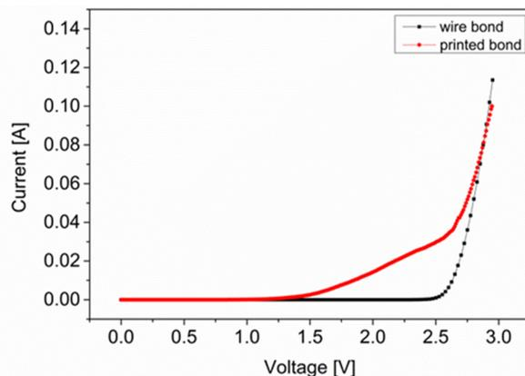
Figure 8: U/I-characteristics of the LED chip with printed dielectrics and interconnects
