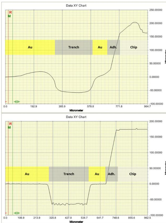
Figure 10: (a) unconnected LED chip (b) Following the top of the silver interconnect with the stylus of a profilometer (Bruker Dektak 150).
