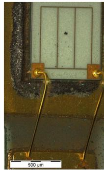
Figure 6: Wire bonded LED chip
