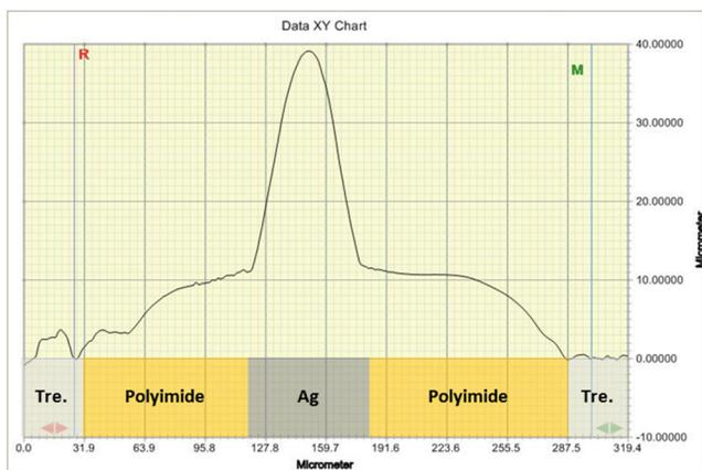
Figure 3: Profilometry image of the printed insulator polyimide and the conductive silver trace on top measured in the isolating trench
