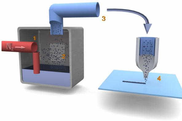
Figure 1. Aerosol Jet® Printing Principle (OPTOMECH, Inc.)
