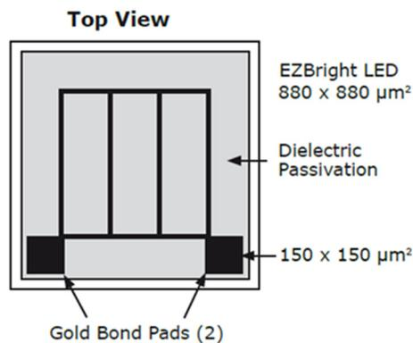
Figure 7: Schematic top view of the LED chip
