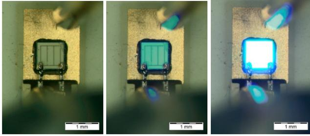
Figure 9: Illuminated LED chip contacted with microprobes.
