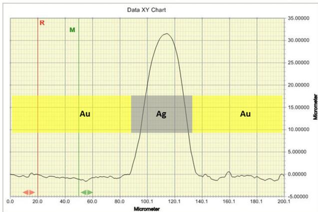
Figure 5: Profilometry image of a silver trace on top of the Au-Pad on the outside of the LED Chip
