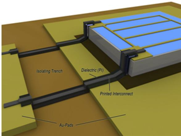
Figure 2: Schematic drawing of printed dielectrics and conductive interconnects of a LED chip using Aerosol Jet® Printing Technology
