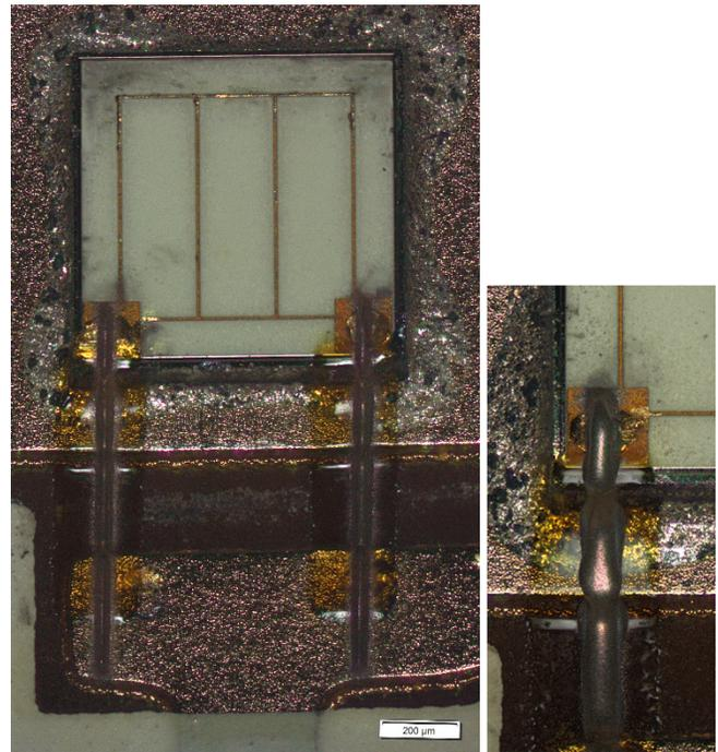
Figure 4: LED chip with dielectrics and electrical contacts by using the Aerosol Jet® Printing Technology
