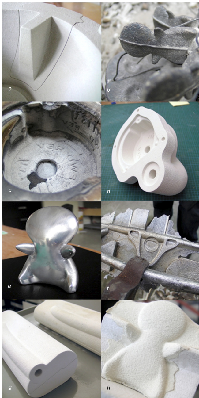
Figure 4 a) detail of slip cast mould's complexity [mechanical fit], b) miniaturized and multiplied objects from original full size file c) detail of metal casting mould interior highlighting heat resistance, d) complexity of mould geometry e) finished aluminum cast from printed mould f) detail of cast skateboard truck immediately after casting [note fin flashing] g) multiple copies of skateboard truck mould prior to casting h) detail of ceramic slip cast on initial mould opening.
