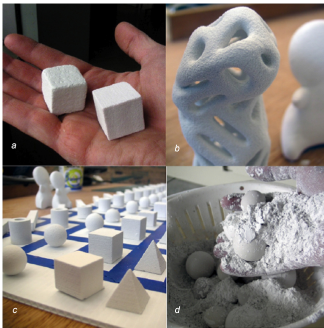
Figure 1: a) Initial comparative tests (L) basic powder formulation (R) commercial powder, b) first "proof of concept" print with new powder formulation, c) selection of iterative tests – closest objects, commercial material, next closest, best formulation of "off the shelf" powder, d) processing powder for uniform consistency.
