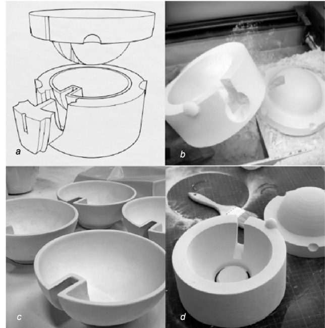
Figure 2 ceramic slip casting: a) digital mould design, b) printed mould being removed from printer, c) ceramic objects slip cast from digital moulds, d) mould components prepped for slip casting.
