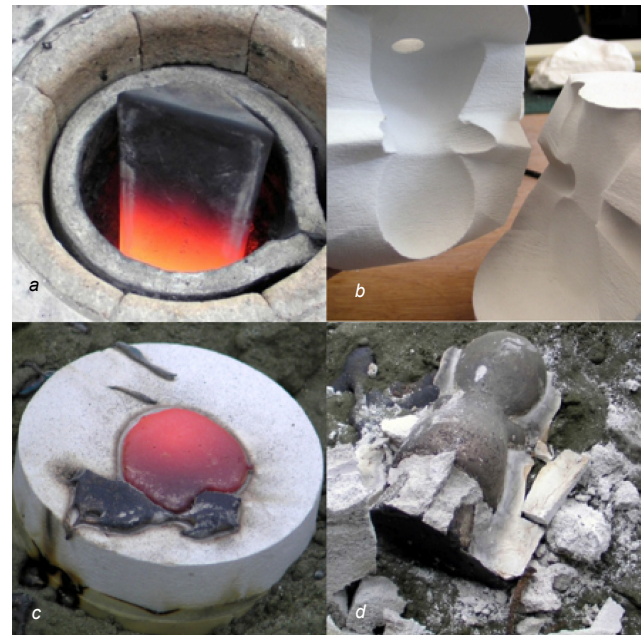
Figure 3 non-ferrous metal casting: a) bronze ingot being melted in induction furnace, b) mould components printed and ready for casting, c) mould soon after being filled with molten bronze, d) removal of mould to reveal cast metal object.
