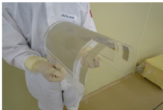
Figure 5 Printed Sample of TFT Array Film
