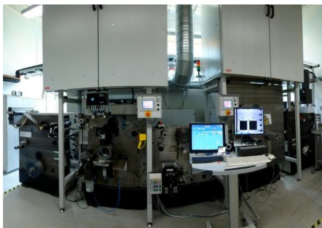
Figure 2: Roll-to-roll rotogravure printing machine LABORMAN from formerly manroland.
