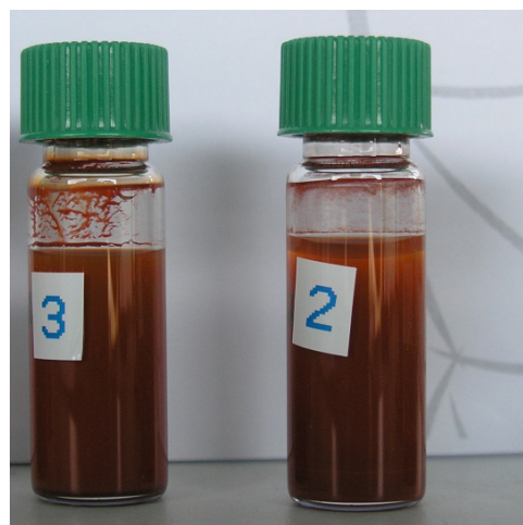
Figure 3 particle loaded inks with stabilizer ethyl cellulose stored for 2 weeks left: 2 wt. % right: 1 wt. %
