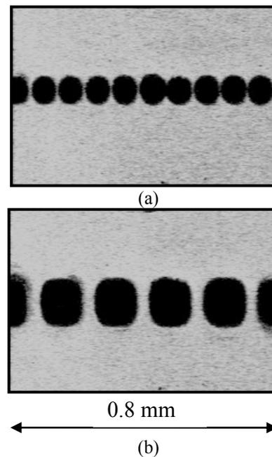
Figure 6. Measurement results of dot patterns formed by scanning laser beam: (a) 1 by 1 and (b) 2 by 2.
