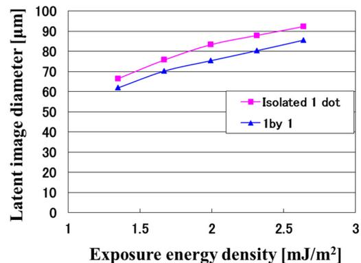
Figure 7. Measurement results of latent image size for dot-patterns.
