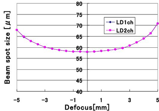
Figure 5. Measurement results of beam spot size of main-scanning direction.
