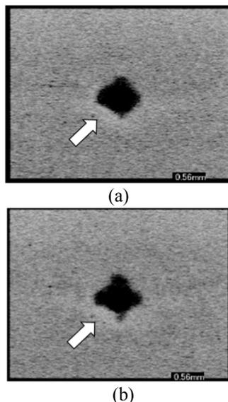
Figure 9. Electrostatic latent images: side-lobe peaks of (a) 7.8% and (b) 12.3% of main-lobe peak. Beam spot size was  $H45 \times 50 \mu\text{m}$ . Charging potential was  $-600 \text{ V}$ .
