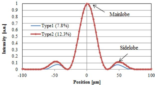
Figure 8. Side-lobe beam profile used for the experiments.
