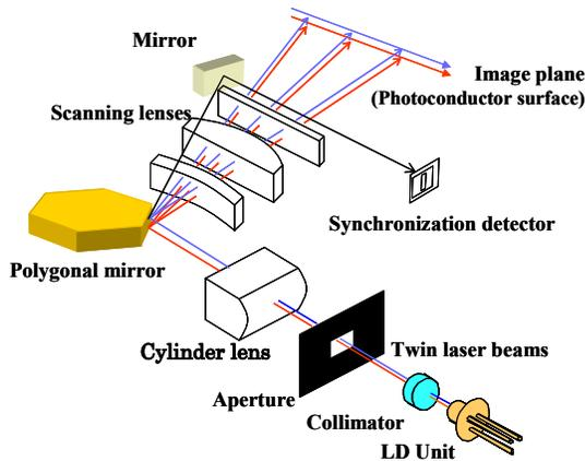
Figure 2. Laser scanning unit (LSU).
