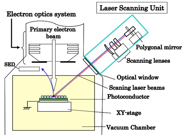
Figure 3. Electrostatic Latent Image Measuring System (ELIMS) equipped with LSU.
