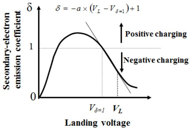
Figure 4. Secondary-electron emission characteristics.
