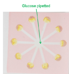
Figure 1. Fluidic channel structure used for demonstrating the glucose sensor. Light pink areas are the printed fluidic channel boundaries. Round areas that are partially red and partially yellow are the reaction spots. In this picture the colour change from red to yellow is not yet complete. The analyte is pipetted at the center of the structure.
