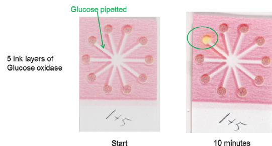
Figure 8. Pilot scale flexography and laboratory scale inkjet printed samples with 5 enzyme ink layers. The glucose is pipetted into one channel and visual colour change can be observed in the marked reaction spot.
