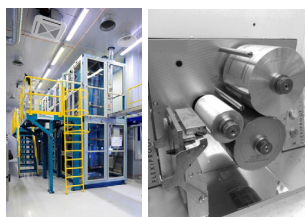
Figure 3. Flexography printing equipment used: pilot scale Maxi printing line at VTT (on left) and laboratory scale RK Flexiproof printer (on right).
