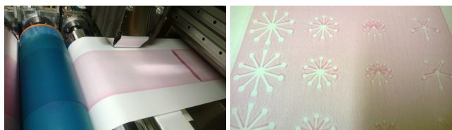
Figure 5. Pilot scale flexography printing of the bottom side of the paper (on left) and final flexography printed top side of the paper that shows how the smallest channels have choked (on right).
