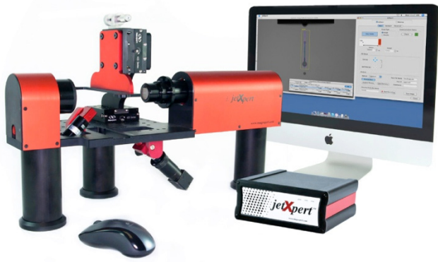
Figure 2 – JetXpert System for Dropwatching and Analysis
