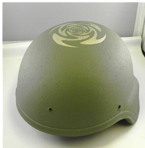
Figure 3. Broadband circularly polarized antenna (2-18GHz) printed on a military-issued combat helmet.
