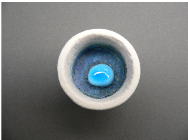
Figure 10. With 5% Copper Carbonate
