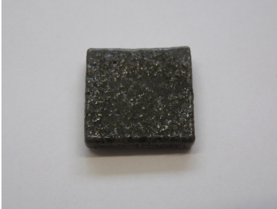
Figure 5. Efflorescence glazed 3D printed tile
