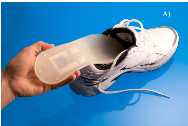
Figure 3 – A) Printed wireless pressure and temperature sensor within a shoe's insole. B) Pressure and temperature data obtained through wireless communication from the printed insole.
