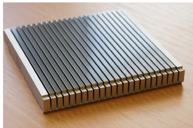
Figure 4 Edge shooter wafer assembly prior to separation
