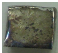
Figure 7. Ag films dipped 10 sec in a 1.0 w/w%, 50 °C aqueous solution of Na_2S
