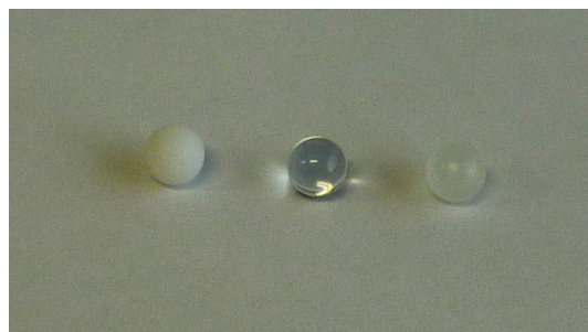
Fig. 4 Photo of balls; from left, PTFE, PMMA, PP ball.
