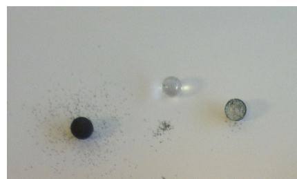
Fig. 5 Photo of balls after mixed with carrier N01; from left, PTFE, PMMA, PP ball.
