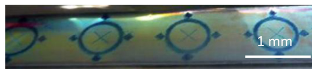
Figure 7. Series of LSMO devices printed onto 10 mm Ni ferromagnetic metallic tape. An epitaxial LZO buffer layer is commercially available on top of this metallic substrate.
