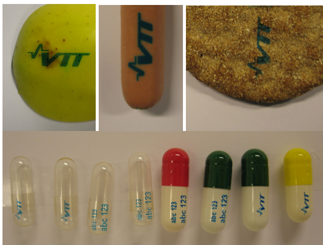
Figure 5. Edible products marked with inkjet printing: on top from left apple, sausage and crisp bread; on bottom medical capsules.
