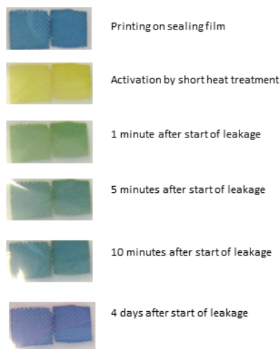
Figure 2. The principle of the developed oxygen indicator.
