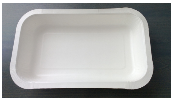
Figure 1. Barrier coated carton board converted into tray package.
