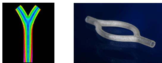
Figure 1. Left: Computational evaluation of shear stress. Right: prototype of an elastic branched tube, fabricated from newly developed cytocompatible ink by UV laser curing.
