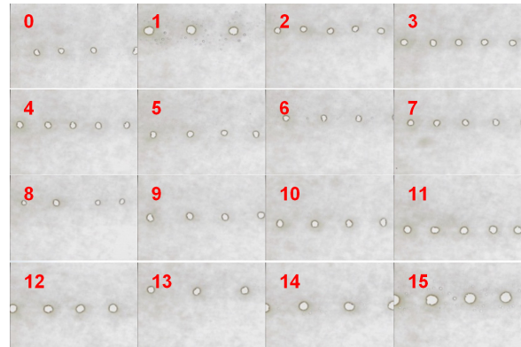
Figure 12. Pulsed jetting with pulse at 2 kHz
