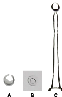
Figure 10. Variations in drop-jet topologies as a function of nozzle geometry: A) standard drop, B) drop with encapsulated bubble, and C) long thin jet.
