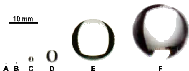
Figure 9. Typical range of auto-ejected droplets in A)-B) in normal gravity, C)-E) in a drop tower, and F) low earth orbit. Droplet volumes vary from A) 0.02, B) 0.06, C) 4, D) 36, E) 1480, and F) 3544 \mu\text{L} .
