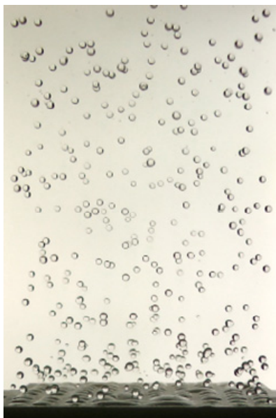
Figure 7. Approximately 300 0.32 \mu\text{L} 1 cS PDMS liquid droplets passively ejected from a 10 by 10 array of tubes.
