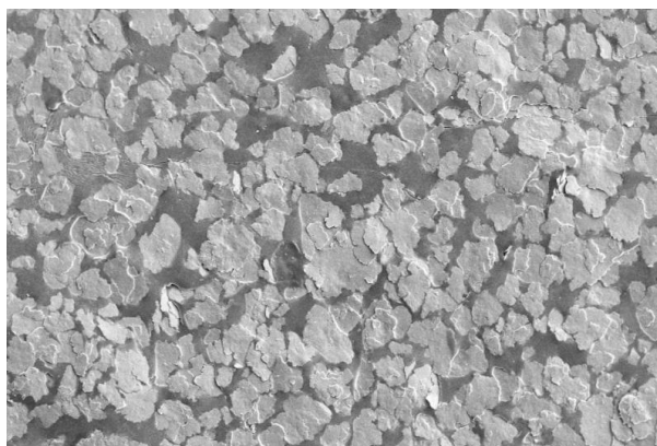
Figure 1: Scanning Electron Micrograph of a fused toner image containing leafing type metallic flakes
