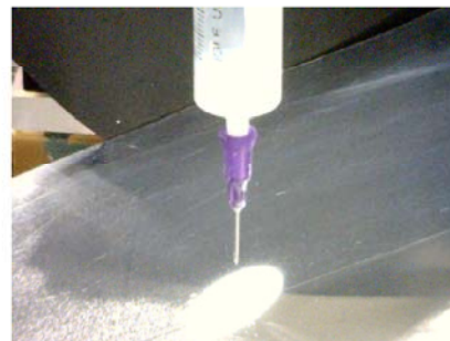
(a-1) printing when the inclination angle is 30 deg.
