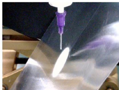
(c)printing when the inclination angle is 60 deg
