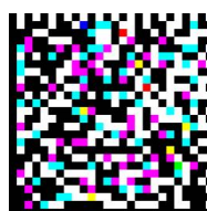
Figure 2. An example progressive barcode using a standard Data Matrix. The black and rest-as-white modules will read using standard Data Matrix software.
