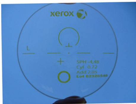
Figure 14. Image printed on pre-cut eyeglass lens with M-series print head.
