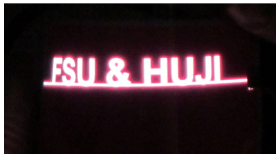
Figure 4. Electroluminescent device prepared by a tailored silver nanoparticle ink and low-pressure plasma sintering. Reprinted from reference 16.
